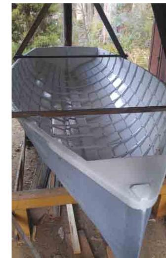
below left: The ribs steam bent and fitted.
