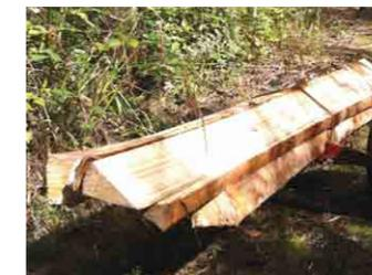
left: Wood split and quartered from a long straight bolt ready to be made into ribs.
