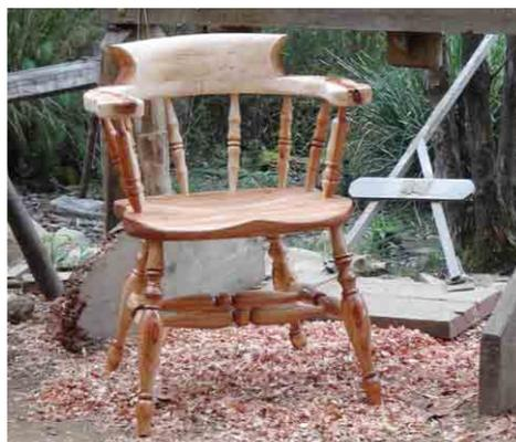
The Captain's Chair will need four legs, four stretchers and eight spindles. The woodworker uses a beetle and wedge to halve the billet and then froe and maul to split each piece in half again and again. This process quickly delivers the necessary raw material. As the pieces reduce in size the froe's accuracy becomes more important – if off centre, the split is unlikely to run straight and the froe will have to be manipulated to steer the split back on course.
